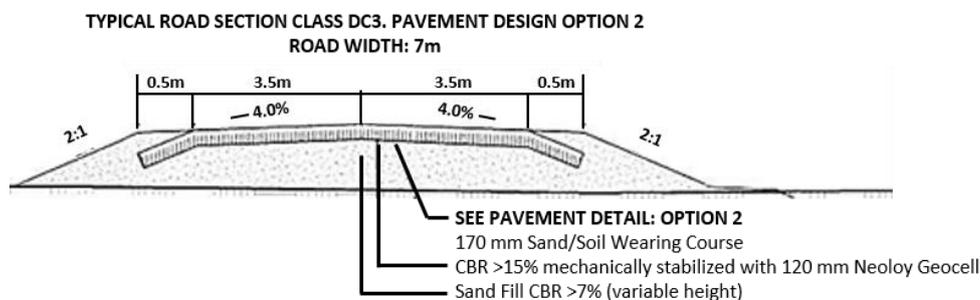
Fig. 3. Typical road section drawing with Neoloy Tough Cell base reinforcement (Source: WSP)
